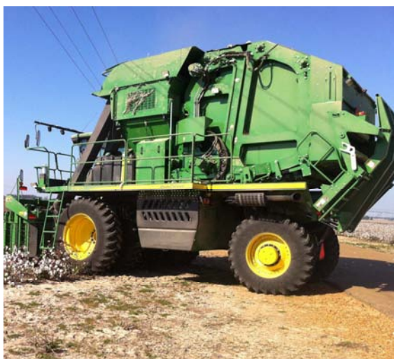
A round bale cotton picker sits at the edge of a cotton field near a round bale. The advantage to round balers is fewer pieces of equipment and less labor needed for harvest.
